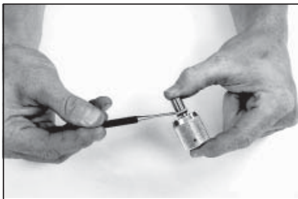
Fig. 5.20 Replace the washer and O-ring if necessary.
