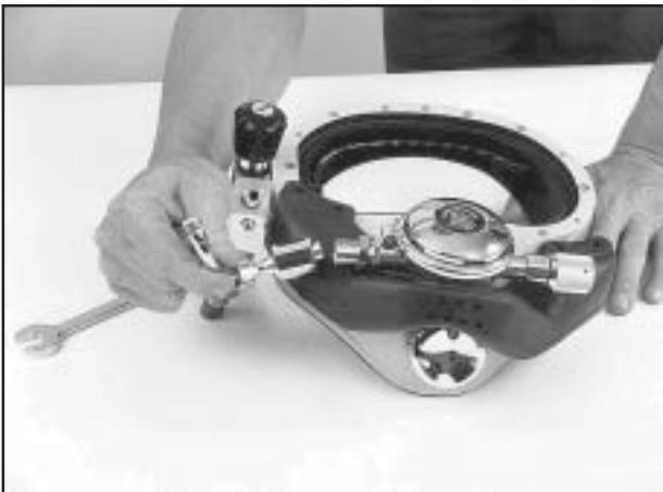
Fig. 6.24 Pull the bent tube assembly straight out of the regulator nipple.
