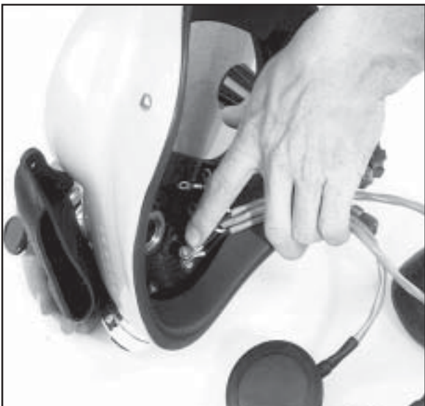
Fig. 6.14 Remove the nut from the communications posts.
