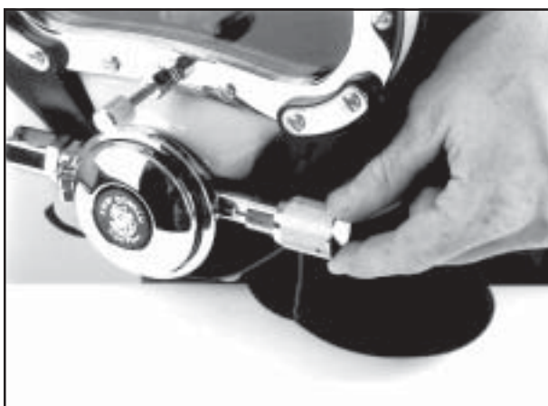
Fig. 6.65 The adjustment knob must turn freely.
