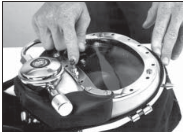
Fig. 6.10 Install the two O-rings on the nose block shaft.
