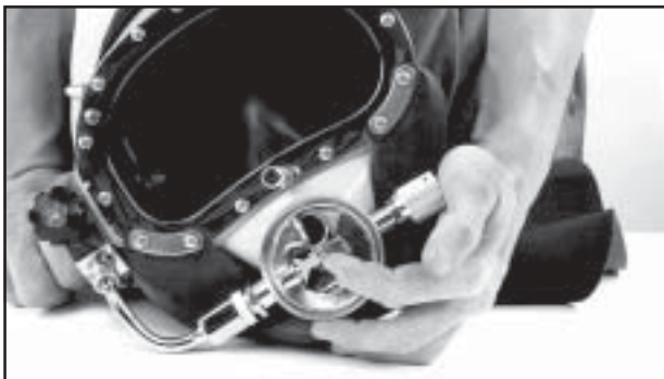
Fig. 5.22 Checking the play in the lever.
