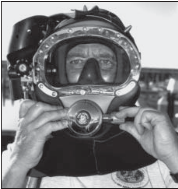
Fig. 2.7 Always test the breathing system prior to diving.
