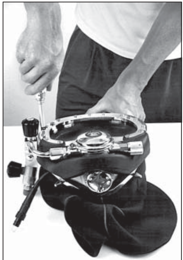
Fig. 6.4 Removing the port retainer screws.
