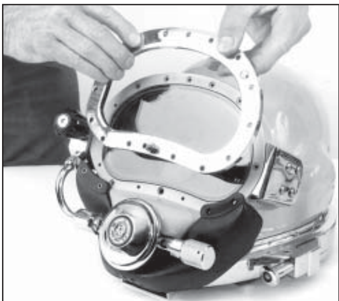
Removing the port retainer.
