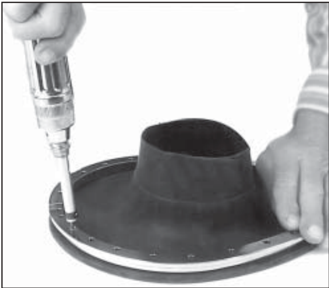
Tighten the screws to 10 inch pounds (12kg.cm.) of torque.
