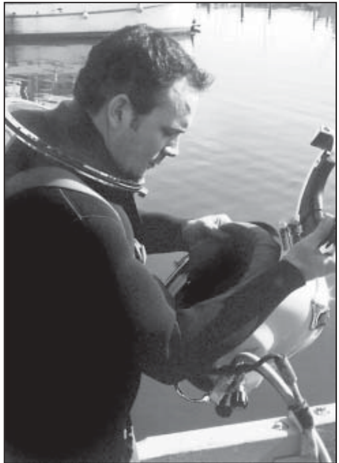
Open the locking collar/neck pad assembly fully.
