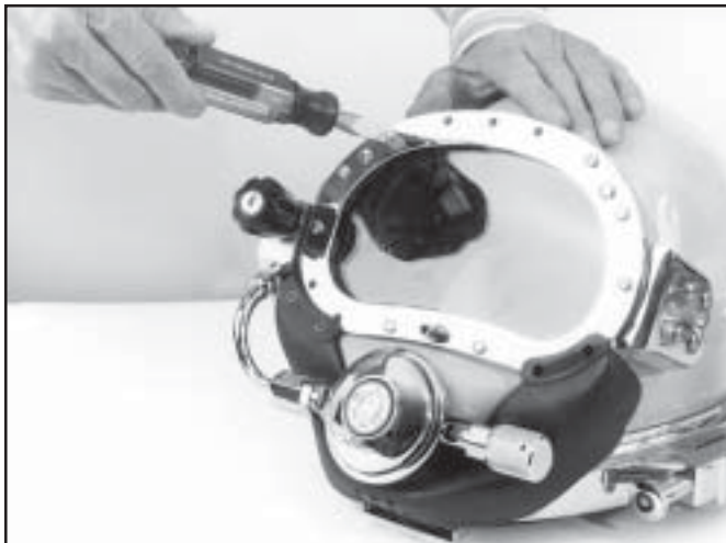
Removing the port retainer screws.
