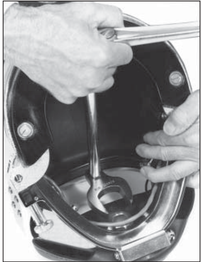
Fig. 6.26 - The regulator mount nut is removed with the proper wrench.
