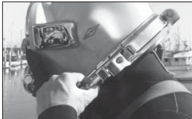
Rotate the sealed pull pins into the locking position.
