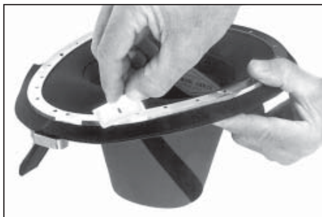
Trim the excess neoprene using a sharp razor
