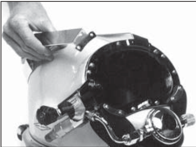
Position the two mount brackets on the helmet
