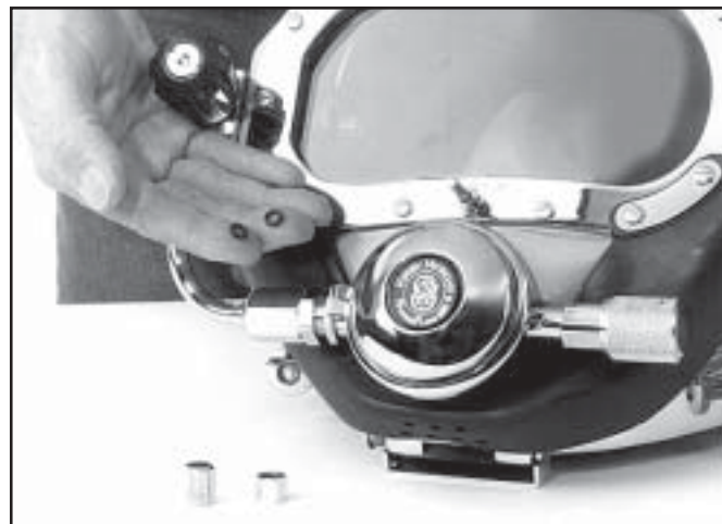
Removing the nose block O-rings.
