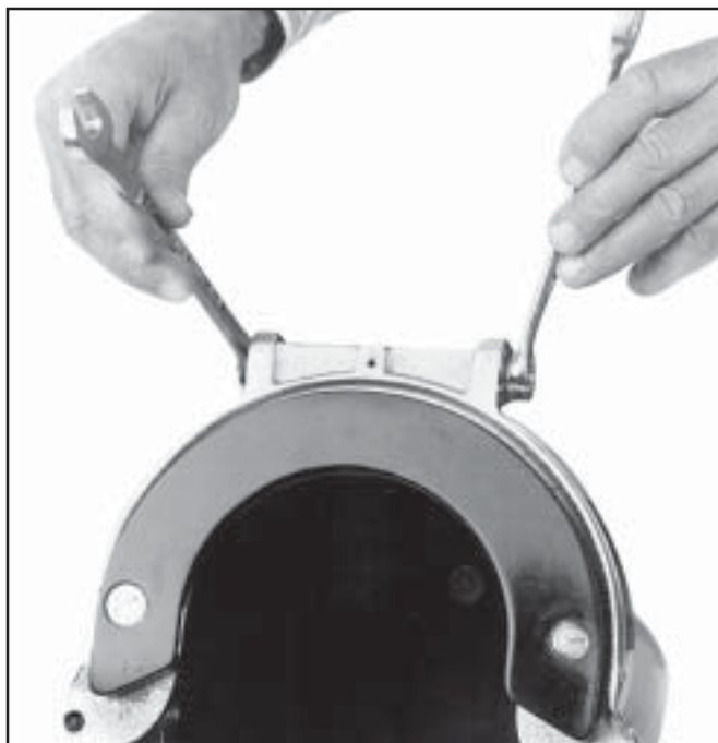
Remove the two bolts from the hinge pin
