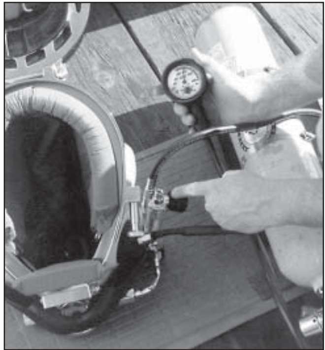
Checking the one way valve.
