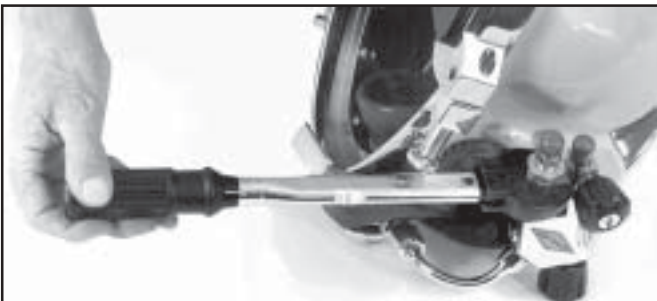
Tighten to 240 inch lbs. (270kg.cm) with a torque wrench.
