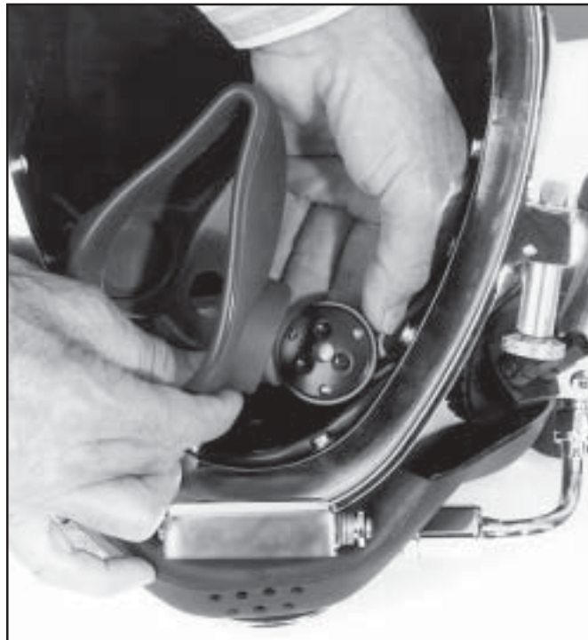
Install the microphone in the oral nasal mask.
