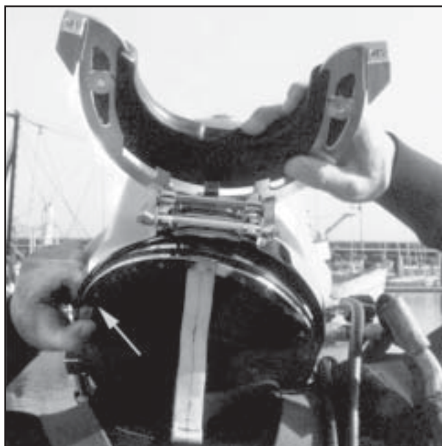
Push the neck dam/ring up into the neck ring on the base of the helmet.
