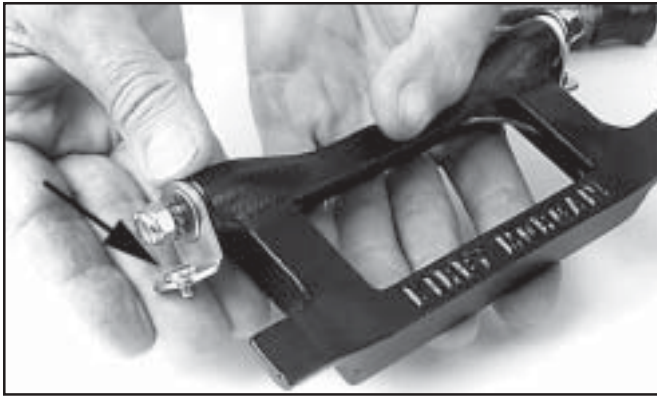
Install the screws through the mount ears.
