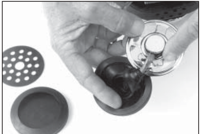
Inspect the mylar earphone.
