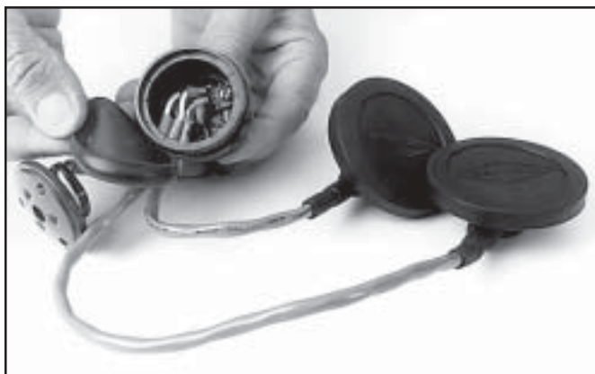
Remove the rubber cover from the communications module.
