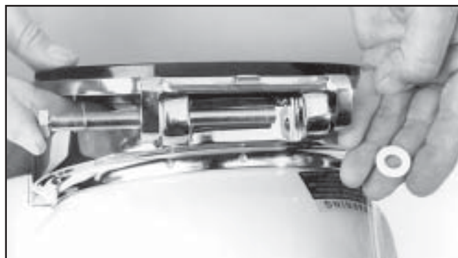
Take care not to lose the two Teflon washers
