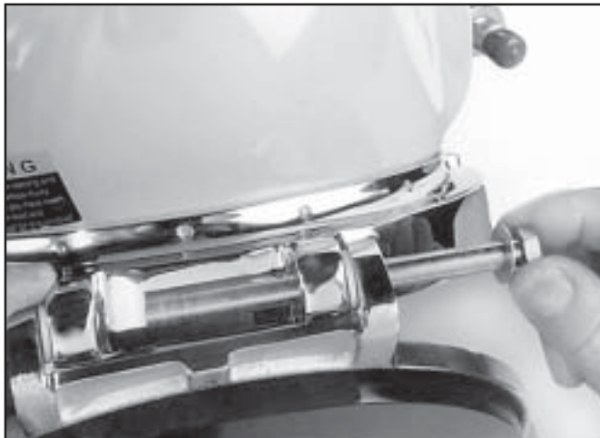
Slide the hinge pin out from the hinge.
