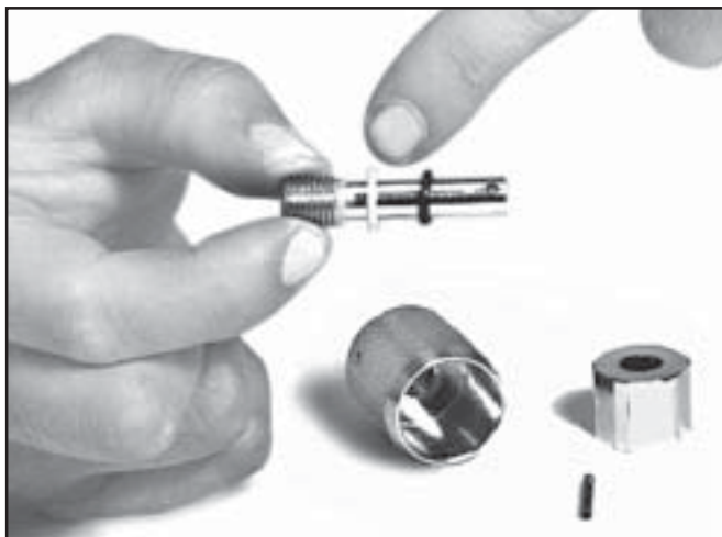
Fig. 6.25 - Inspect the O-ring & washer.
