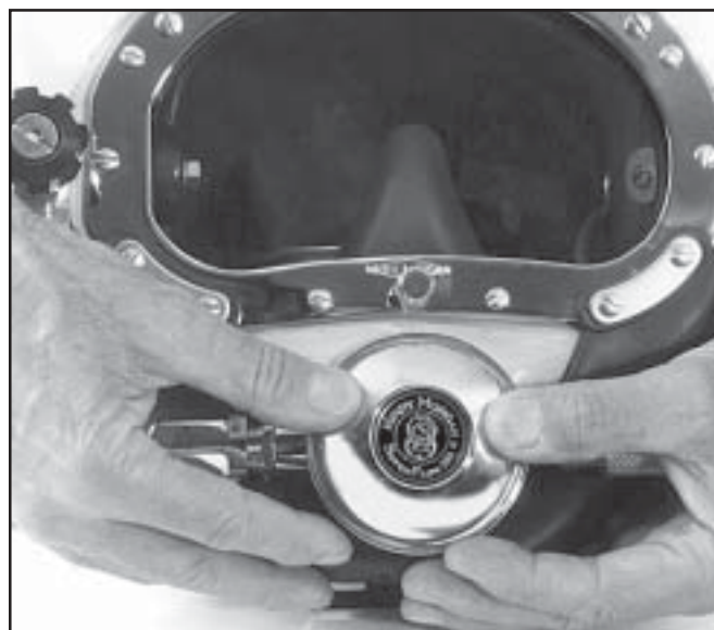
Press the cover over the diaphragm.
