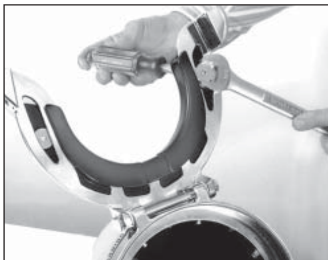
Unscrew the two screws that hold the neck pad.
