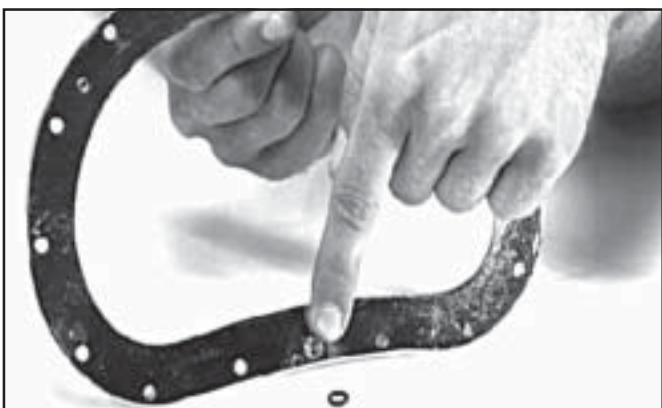
Be sure to install the O-ring on the back of the port retainer.
