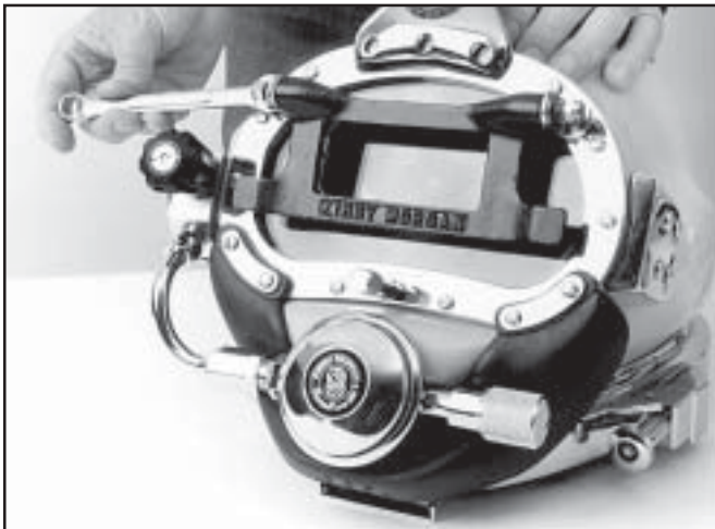
Tighten the weld lens assembly.
