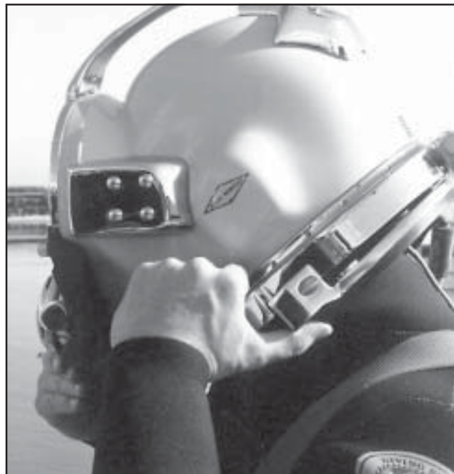
Both sealed pull pins must properly click into position on the base of the helmet.
