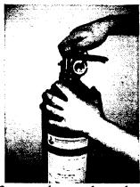
13. screw the complete valve assembly back into the cylinder. Turn the extinguisher upside down a few times to ensure a good mixture.
